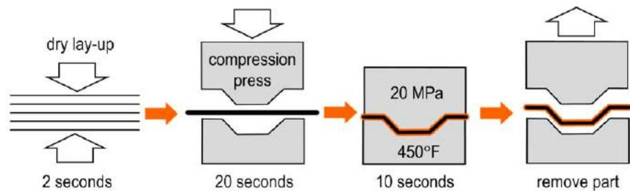
Figure 3. High speed consolidation and molding for Malleable materials
