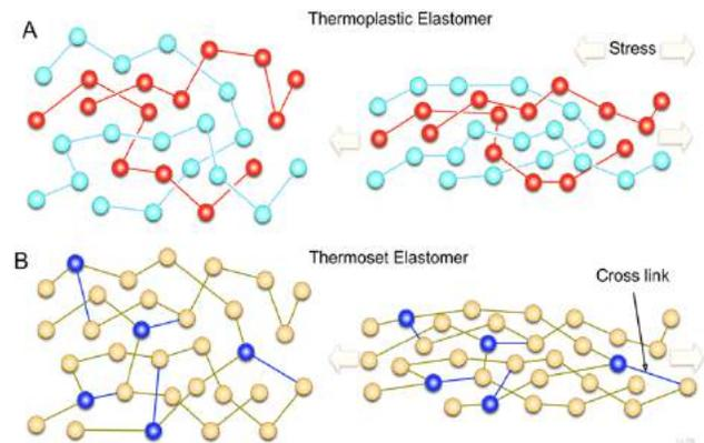
Figure 1. Thermoplastics vs. Thermosets
