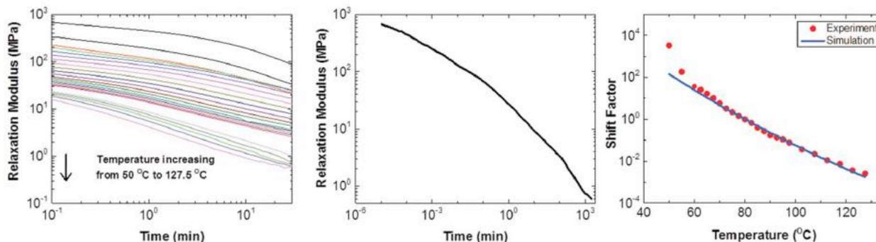
**Figure 2.** Temperature-dependent stress relaxation behavior of vitrimers shows that malleable flow of vitrimers correlates with reaction-rate of bond exchange.
