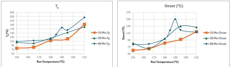
Panel curing example: out of autoclave cure of 10 ply panel: vacuum bag, in oven, 135°C 40 min, 180°C 2h. After cure press: 30psi 190C, 30 minutes, cool to 60C remaining at 30psi. *result: T<sub>g</sub> 128°C, Onset 105°C.*
