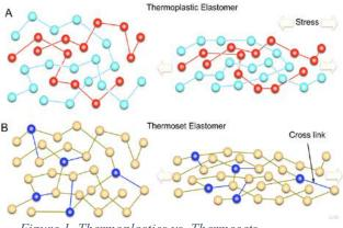
Figure 1. Thermoplastics vs. Thermosets
