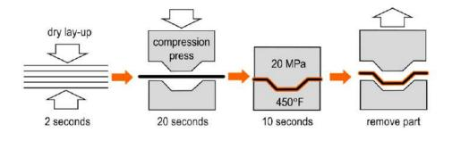
(rather than *Figure 3. High speed consolidation and molding for Mallinda's malleable materials* estimated) fiber/resin
