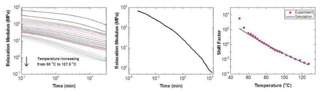
**Figure 2**. Temperature-dependent stress relaxation behavior of vitrimers shows that malleable flow of vitrimers correlates with reaction-rate of bond exchange.
